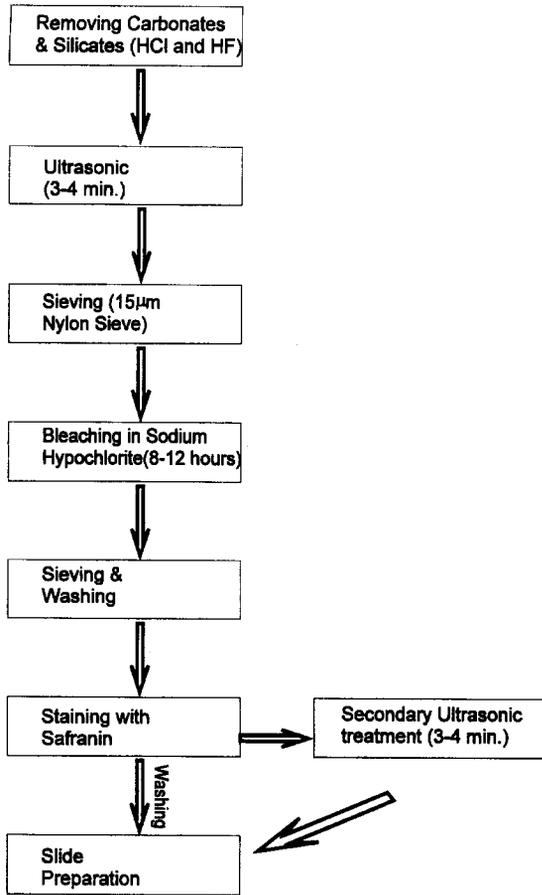
Fig. 2. Sample preparation procedures in the proposed bleaching method.
